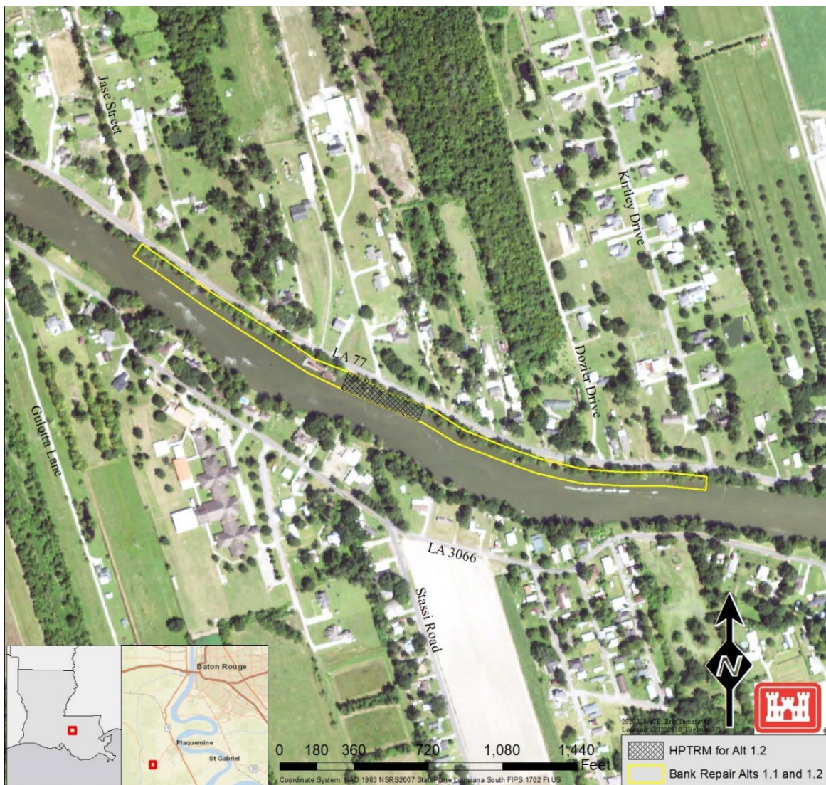
Figure 1: Proposed repair reach and Alternative Design Options 1.1 and 1.2
